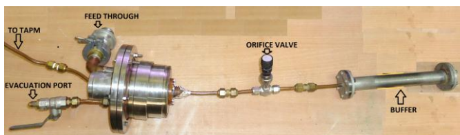
Figure 3. Photograph of Pulse Tube Refrigerator
