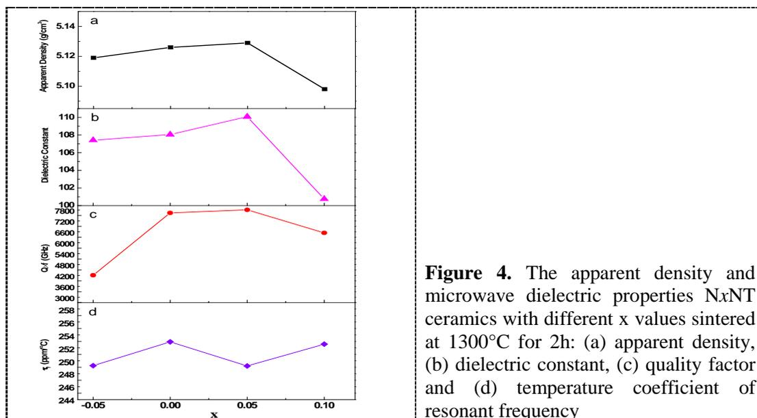
**Figure 4.** The apparent density and microwave dielectric properties  $N_xNT$  ceramics with different  $x$  values sintered at  $1300^\circ\text{C}$  for 2h: (a) apparent density, (b) dielectric constant, (c) quality factor and (d) temperature coefficient of resonant frequency
