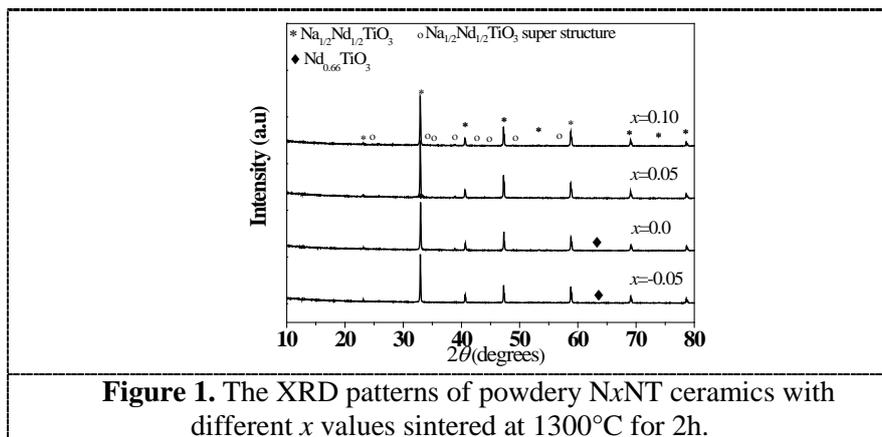
**Figure 1.** The XRD patterns of powdery  $\text{NxNT}$  ceramics with different  $x$  values sintered at  $1300^\circ\text{C}$  for 2h.
