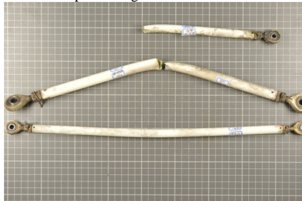
Figure 2. Fractured and bending connecting linkage
