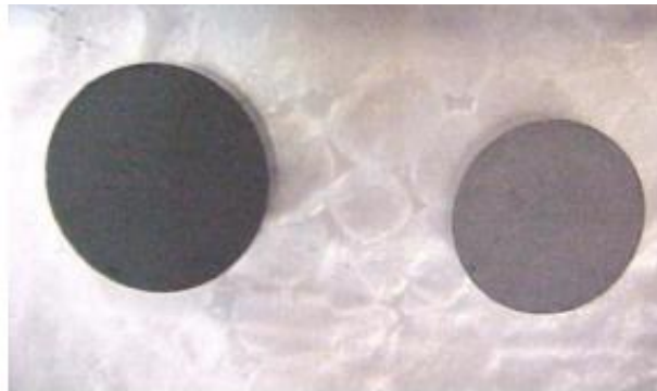
Figure 4: Photographs of the WC-12Co compacts derived from microcrystalline powders after microwave sintering in a 90N 2 -10H 2 atmosphere, before (left hand side) and after (right hand side) sintering [71].
