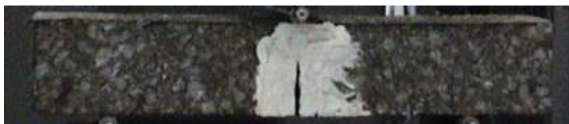
Figure 4. 3-point bending specimen.
