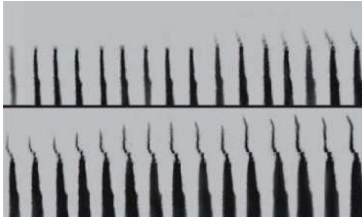
Figure 2. Crack propagation process.
