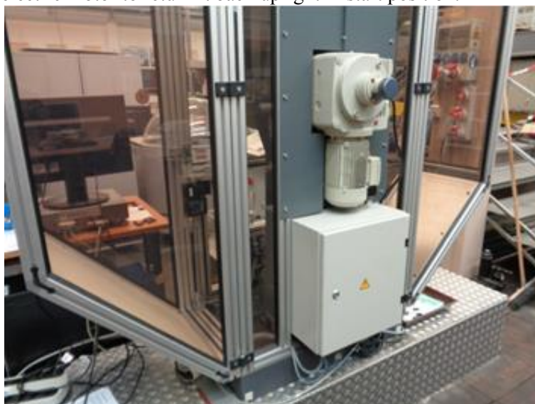
Figure 5. Electric motor and gear box, Laboratory Hochschule Ulm, Germany
