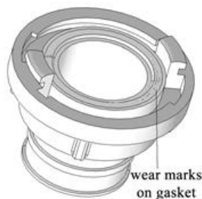
Figure 6. Wear of the sealing gasket
