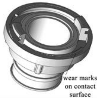
Figure 7. Wear marks on the flanges
