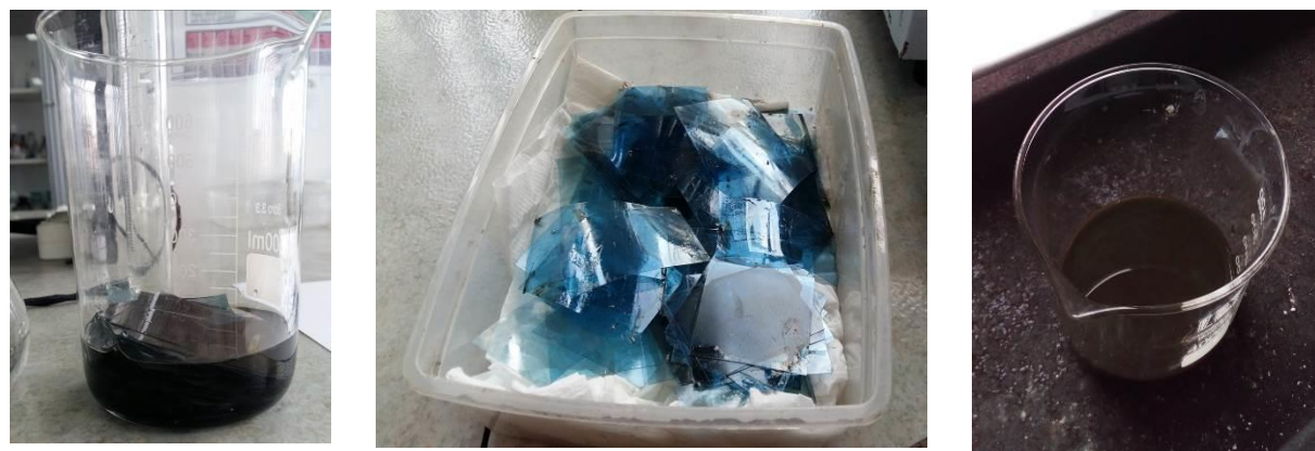
Figure 4. The leaching, the extraction of the clean film, the evaporation of the liquid phase
