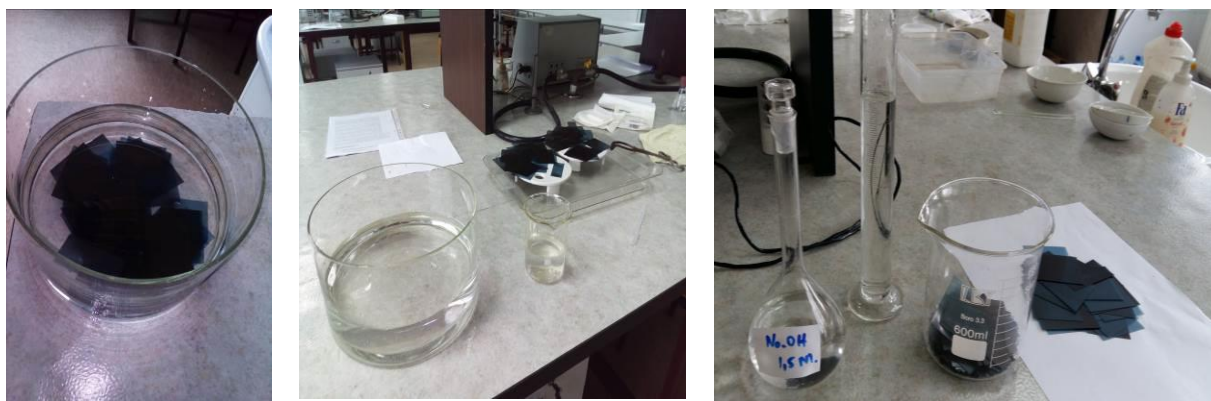
Figure 3. Radiographic film preparation (washing, drying, treatment with NaOH 1.5M)
