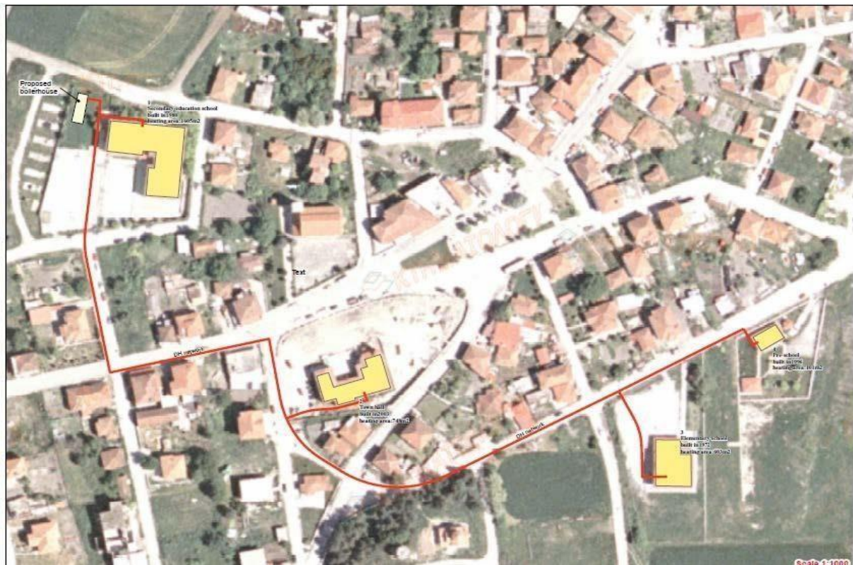
Figure 1. Configuration of the biomass district heating system of Karpero.
