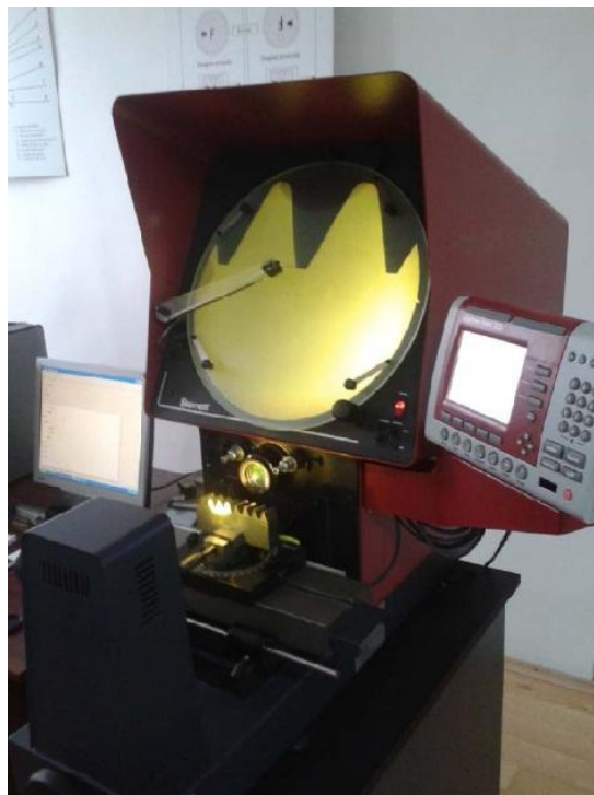
Figure 3. The real rack-gear flank's measuring.
