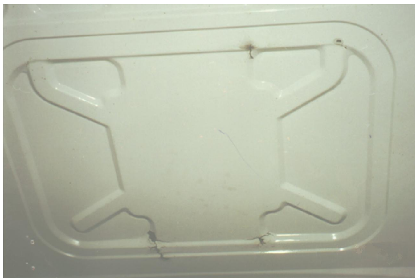
Figure 1. The cracks observed on the roof panel
