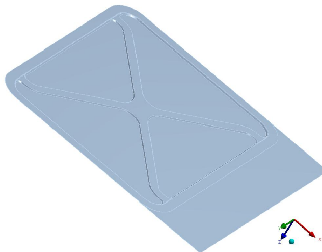
Figure 6. Proposed model with X-shape ribs
