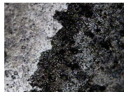
Carburized Steel (950°C)
