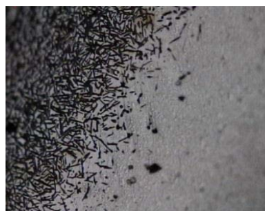
Carburized steel (900°C)
