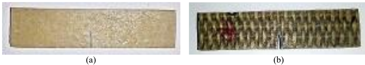
Figure 2. Pre-notched samples (a) virgin polyester and (b) 0/90/0/-90/0 fiber orientations.
