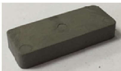
Figure-3. Injected Sample for Solvent Debinding
