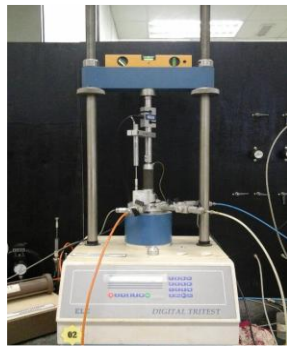
Figure 2 Unconfined Compressive Strength Test Equipment
