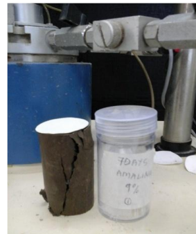
Figure 3 Unconfined Compressive Strength Typical specimen
