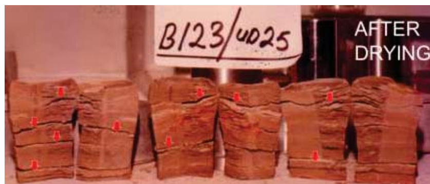
Figure 5 Clay portion will shrink exposing discontinuities
