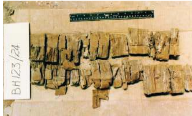
Figure 6 Undisturbed samples taken from a borehole
