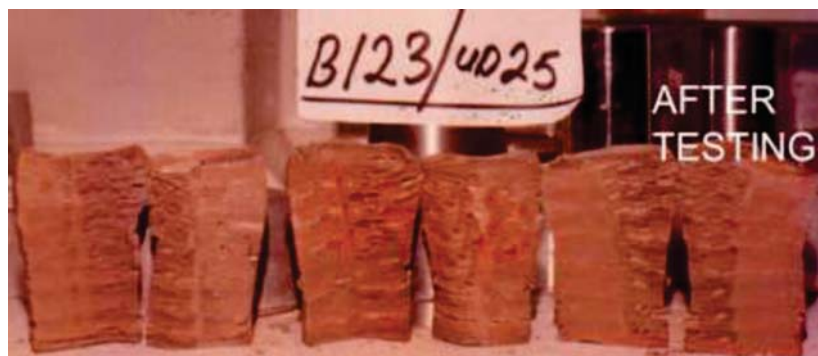
Figure 4 Undisturbed samples cut open after testing
