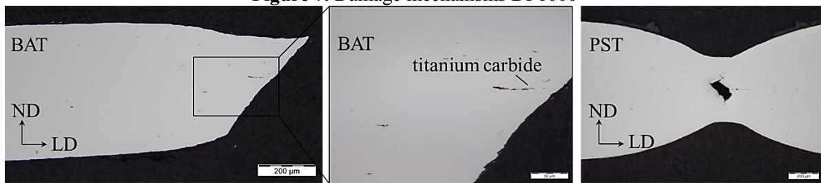
Figure 8. Damage mechanisms CP1000
