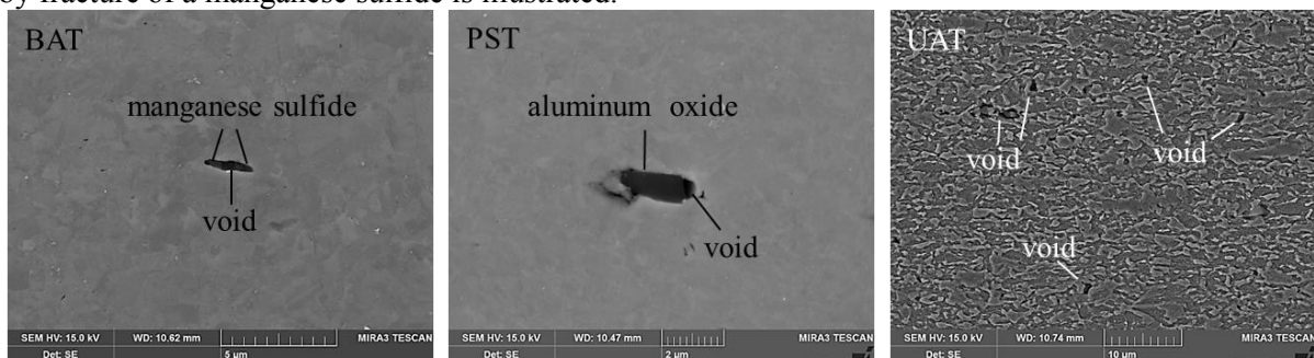
Figure 5. Damage initiation DP1000
