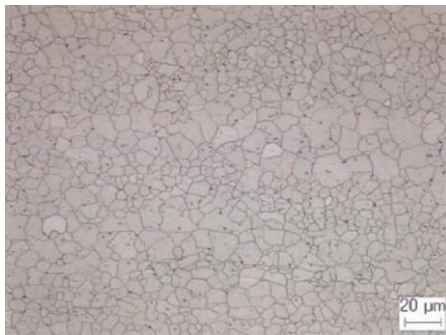
Figure 1. Optical microscopy of the as-received AZ31B sheet
