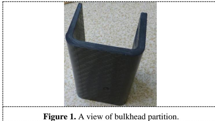
**Figure 1.** A view of bulkhead partition.
