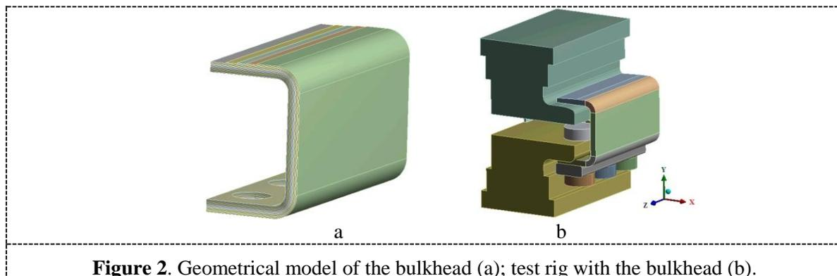
**Figure 2.** Geometrical model of the bulkhead (a); test rig with the bulkhead (b).
