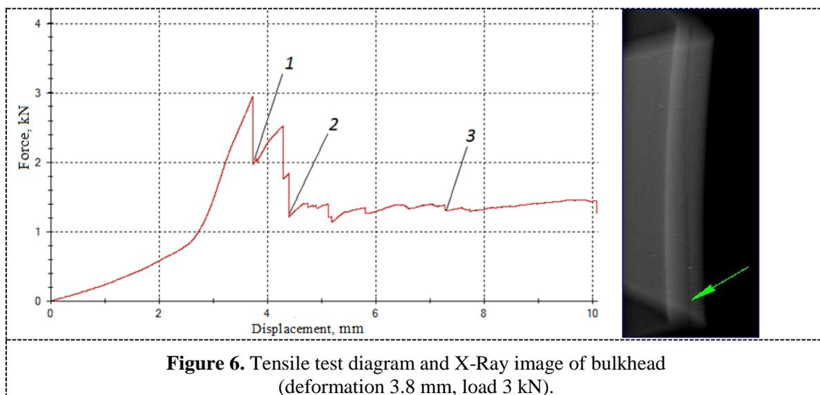
**Figure 6.** Tensile test diagram and X-Ray image of bulkhead (deformation 3.8 mm, load 3 kN).
