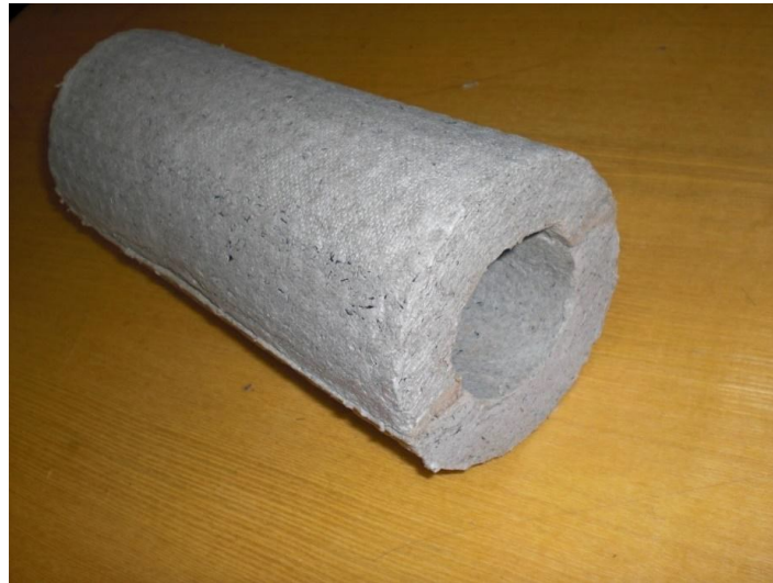
Figure 9. View of the assembled heat insulation basalt shells for rockets and spacecraft
