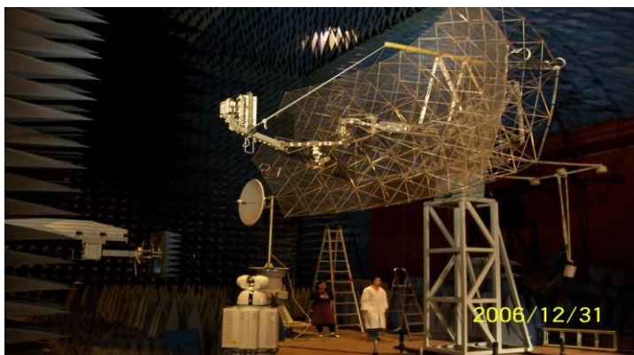
Figure 2. Mesh reflector of the space antenna during ground tests (JSC “OKB MEI”, Russia).
