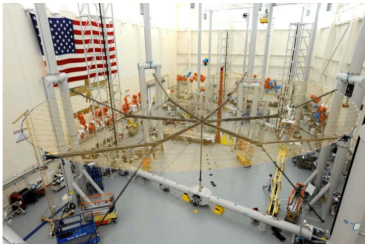
Figure 3. Deployed TerreStar-1 18m reflector at Harris facility.
