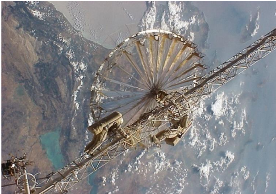
Figure 1. Mesh reflector prototype during orbital testing at the Mir space station (JSC NPO “EGS”, Russia – Georgia).
