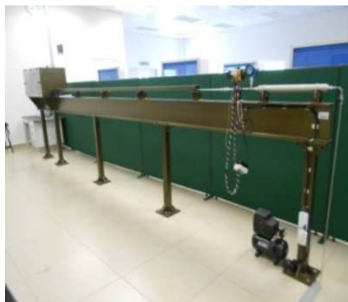
Figure 3. Single Stage Gas Gun (SSGG)
