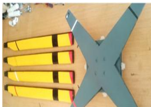
Figure 7. Prototype of main rotor hub and blades
