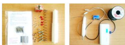
(a) (b) Figure 8. (a) SMA actuators and power supply and (b) ARBF assembly
