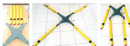
(a) (b) Figure 8. (a) SMA actuators and power supply and (b) ARBF assembly
