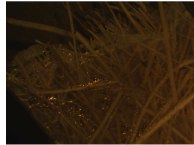
Figure 9. Microscopic image (magnification 200MP) of the fractured surface after the flexural test of palmyra waste fiber (30% wt) and coir fiber (70% wt) of fiber length 4 cm hybrid composites
