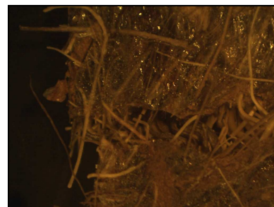
Figure 3. Microscopic image (magnification 200MP) of the fractured surface after the tensile test of palmyra waste fiber (50% wt) and coir fiber (50%wt) of fiber length 4 cm hybrid composites
