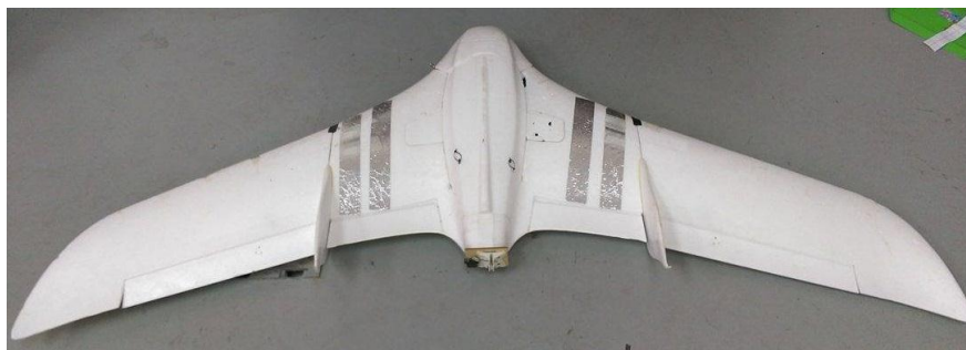
Figure 3. FX79 fixed wing with 2 m wingspan
