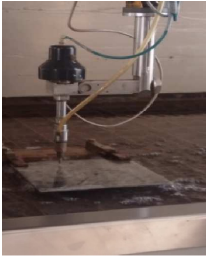
Figure 2. Water jet cutting process of the specimen
