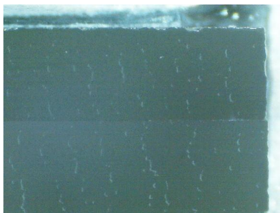
Figure 4. Coarseness and surface pattern of single crystal after polishing by ASM 0.5/0 suspension on VeTex polisher (magnification \times 50 ).
