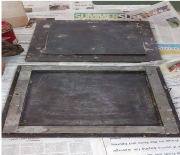
(a) Thin layer of PVA coated dies
