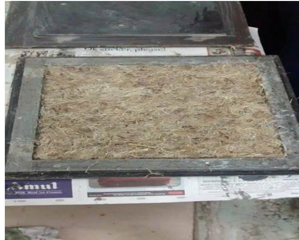
(b) Mixture of matrix and reinforcement filled in die
