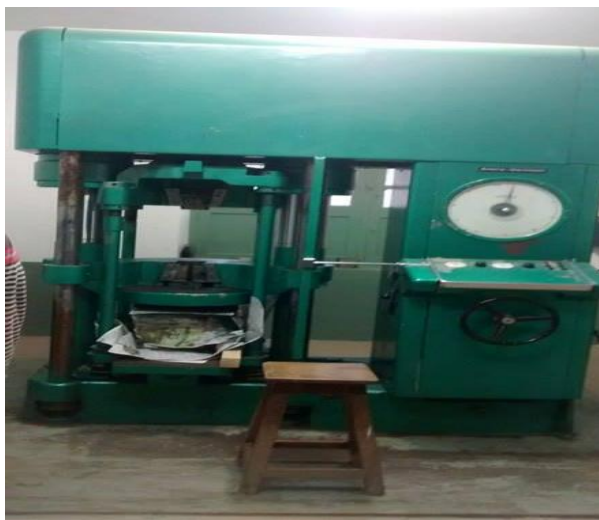
(c) Die pressing by Hydraulic pressing machine
