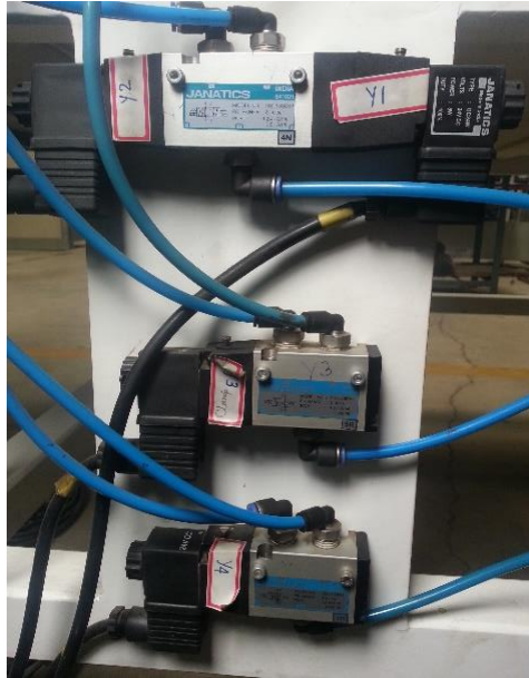
Figure7(b): Fabricated pneumatic circuit
