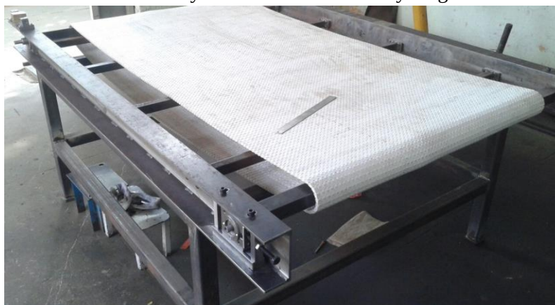
Figure:6 Conveyor mounted on the shaft
