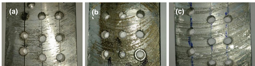
Figure 6. Burr heights observed on drilling of (a) Base Alloy (b) Mono alloy and (c) Hybrid alloy with TiN coated HSS, M42 and carbide drill bits
