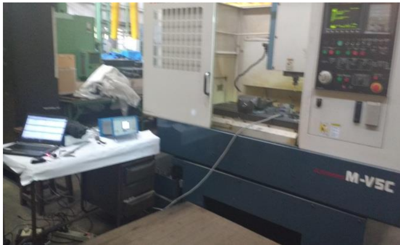
Figure 2. Experimental setup with drill tool dynamometer and DAQ system
