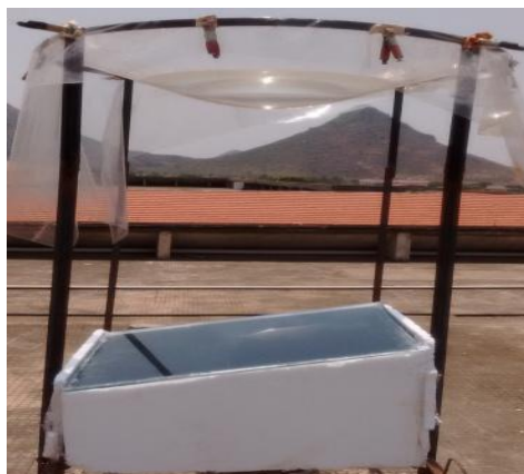
Figure 4. Experimental setup of single slope solar still with insulation
