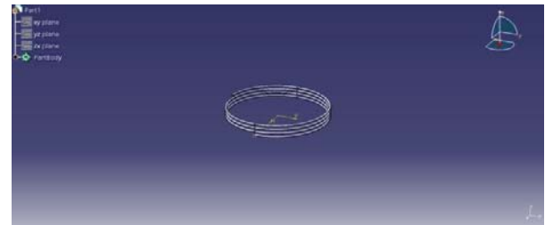
Fig 4: Capillary tube of the vapor compression refrigerator
