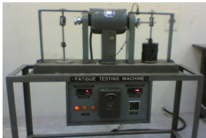
Figure 3. Fatigue testing machine.
