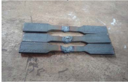
Figure 1. Weld specimens prepared using plasma arc welding
