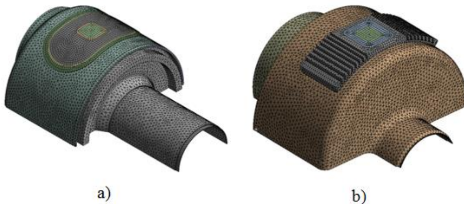
Figure 4. Mesh models (a) Base design and (b) Concept design
