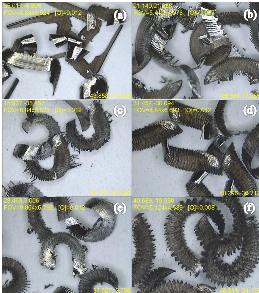
Figure 7. Chip morphology under various conditions (a) Dry cut 75m/min (b) Dry cut 100m/min (c) MQL with air 75 m/min (d) MQL with air 100 m/min (e) MQL with oxygen 75 m/min (f) MQL with oxygen 100 m/min.
