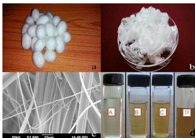
Fig. 2. Formation of AgNPs a) Cocoons b) Silk fibroin fibers c) SEM image of silk fibroin fibers d) Colloidal SF-AgNPs.
