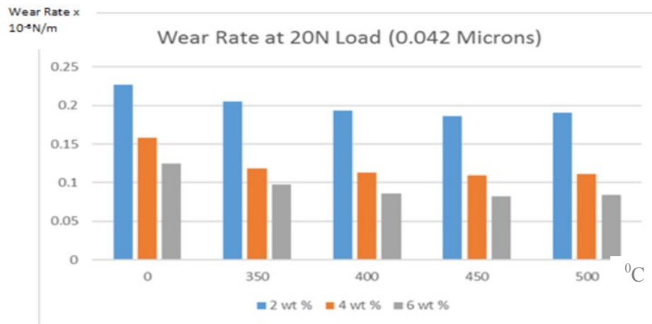
Figure 7. Plot between wear rate and % weight fraction of red mud (0.042 \mu\text{m} ) with aluminium and tungsten carbide and temperature at 20N load
