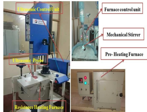
Figure1(b). Ultrasonic assisted stir casting setup
