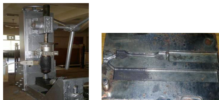
Figure 2. Injection moulding machine along with mould
