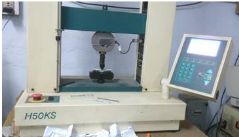
Figure 5. UTM (Hounsfield) machine with bending test fixture
