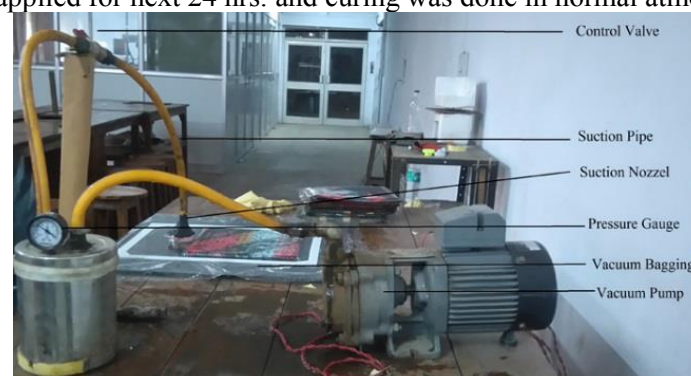
Figure 3. Vacuum bagging set-up
