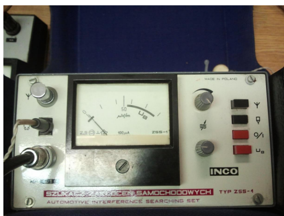
Figure 7. The finder of electromagnetic interference type ZSS-1.
