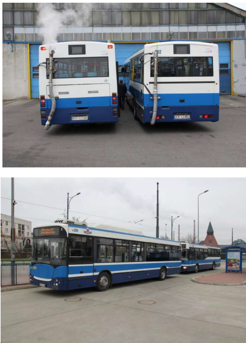
Figure 2. View of tested buses (bus with engine powered by CNG– left, bus with engine powered by diesel – right).
