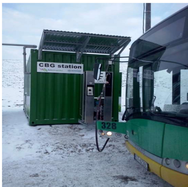
Figure 1. The view of the mobile installation for biogas upgrading, compression, storage, and distribution of biomethane in Poland.
