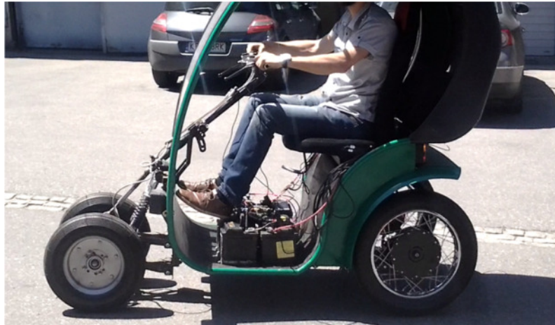
Figure 5. MIST microcar equipped with measuring set.
