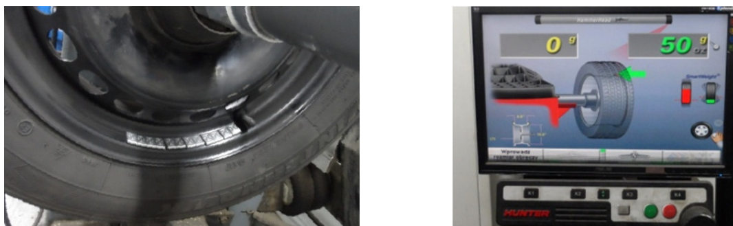
Figure 3. View how to place weights on the rim to the wheel unbalance and a view of the computer screen devices Hunter GSP 9700.
