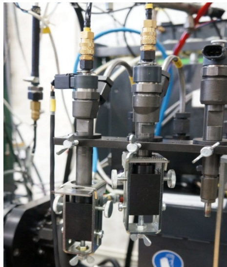
Figure 3. A view of injectors mounted in test chambers [1]
