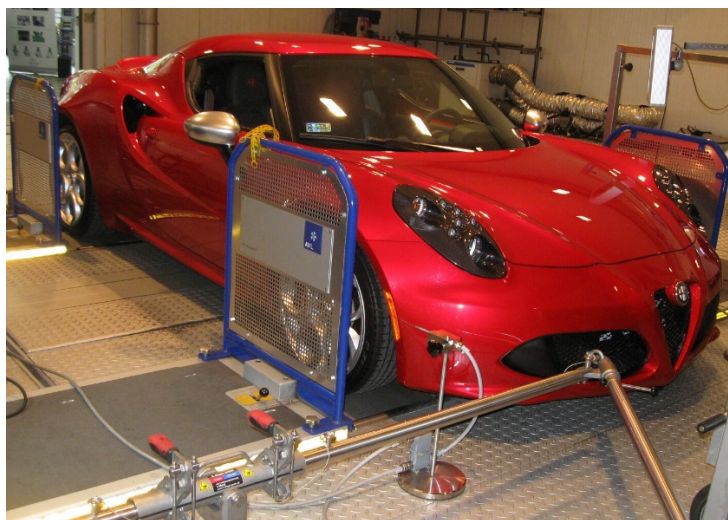
Figure 3. BOSMAL Emission Testing Laboratory – internal view of the climatic chamber.
