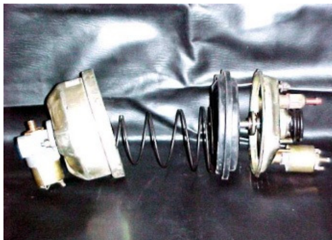
Figure 1. Vacuum servo-motor of automatic clutch [2].
