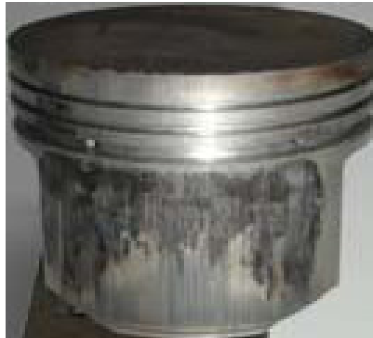
Figure 1. Traces of galling of the guide surface of a piston.
