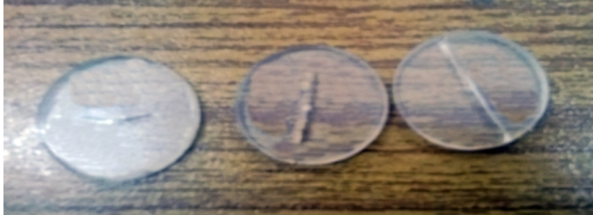
Figure 1. Indentation in Plexiglas with the conical indenter showing well defined radial cracks
